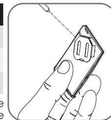
2. Use finger nails to separate the remote casing to expose circuit board.
