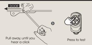
CAUTION: Do not use the string handle as a mechanism to open the door. Failure to comply may cause serious injury.
